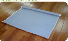
Thickness 0.45mm Weight 520g ∕ m<sup>4</sup> Width 960mm x Length 30M ∕ roll Color Grey Heat resistant temperature Glassfiber cloth appox. 300°C Silicone resin approx. 200°C As spark-protection sheets, heat-resista nt curing covers and heat-resistant par tition sheets
